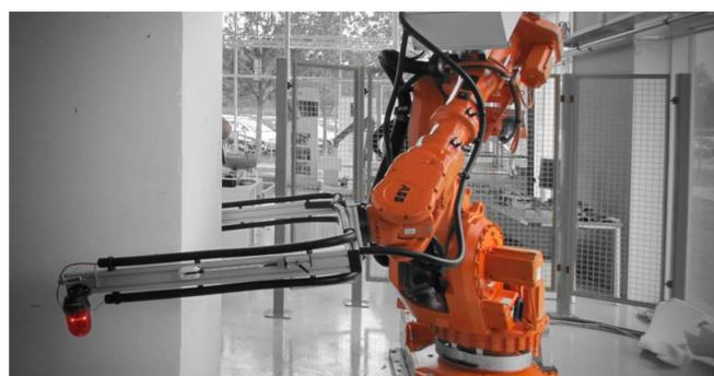
Robot cutting styrofoam block using HotWire.
